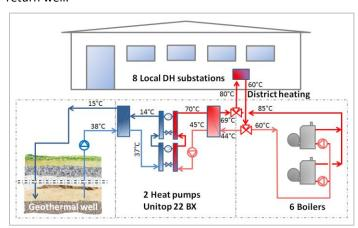
The Loup Pendu - district heating station of Plessis-Robinson draws the energy needed through two closed loop wells from the Neocomian aquifer at a depth of 850m. The supply well is located next to the machine room. Hydro-cyclonic filters remove sand and other solid matter with very little head loss. The reinjection well is located 900m downstream of the supply well.
